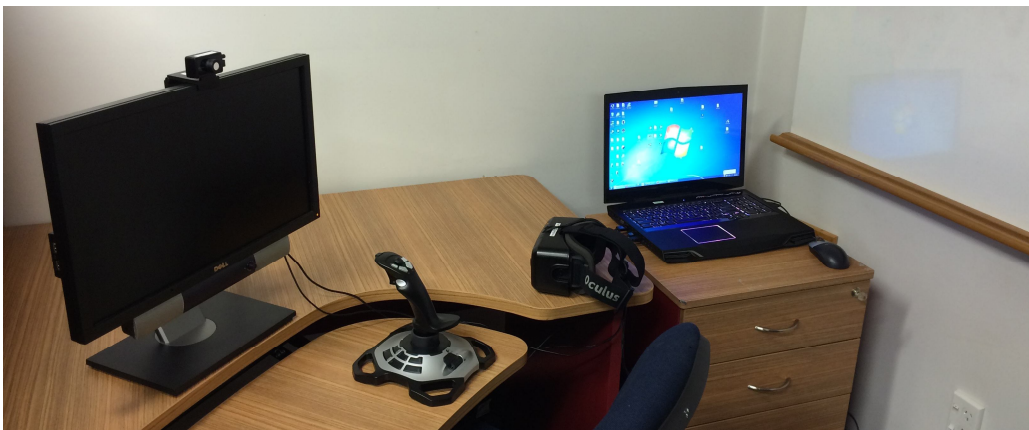
Figure 3: Experiment components including monitor, joystick, HMD, laptop, and HMD tracker placed at the top of the screen
